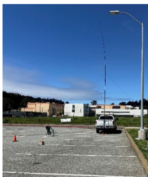
KJ6TSX antenna setup 66-foot End-Fed 40, 20, 15, & 10-meter bands
